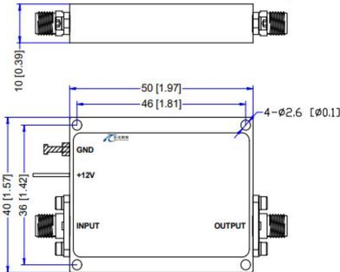
**\*\*\*Heat Sink Required During Operation**
